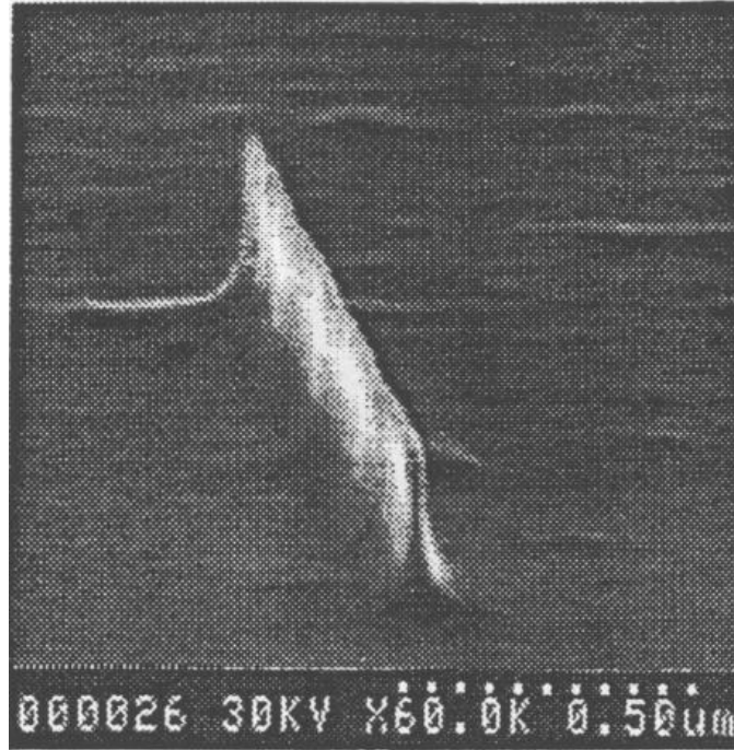
Quantum wire (width 20 nm)
